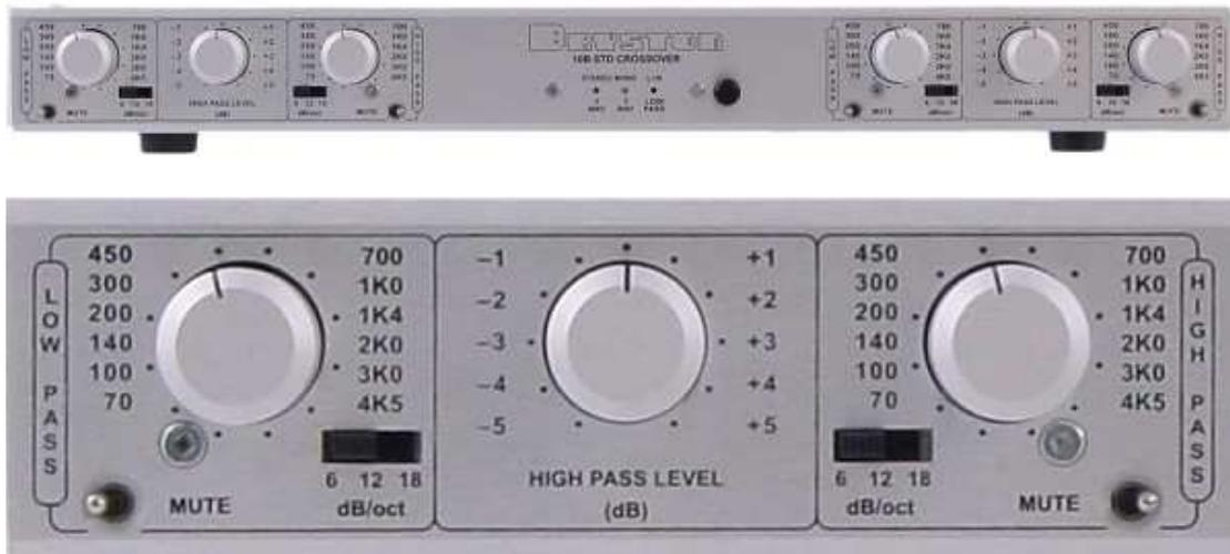
You can see on the front panel in the photo above that there are three sets of control knobs on the left and on the right. The first one on the left controls the low-pass frequency, and there is a slider switch nearby to select the slope (6 dB, 12 dB, or 18 dB per octave). The second knob from the left is an attenuator for adjusting the output of the high-pass section, and the third knob selects the high-pass crossover frequency, with a slope selector underneath.
